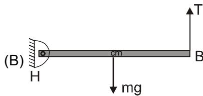
Applying torque balance about the hinge point 'H'
